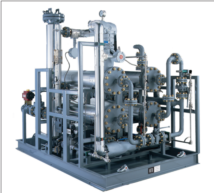
Figure 6. A photograph of a gas turbine conditioning unit. This compact unit has the dimensions 8 ft long X 6 ft wide x 6 ft high and can process up to 1.5 MMSCFD of fuel gas.
